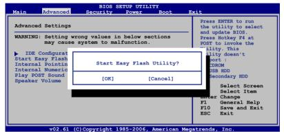
4. Locate the latest BIOS file and start updating (flashing) the BIOS.
